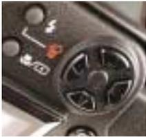
The rear-mounted rocker switch makes menu navigation easy
